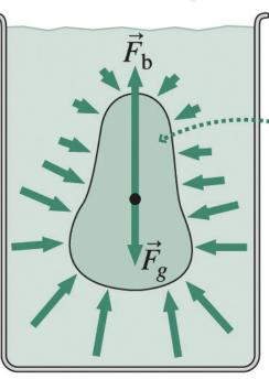
Replace the fluid with a solid object, and the pressure force doesn't change. But the weight may.
