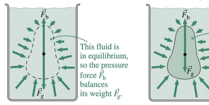
Replace the fluid with a solid object, and the pressure force doesn't change. But the weight may.
