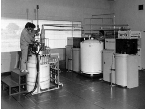
Figure 11.3.4. 17.5 T superconducting magnet system operated at the National Research Institute for Metals. 15
