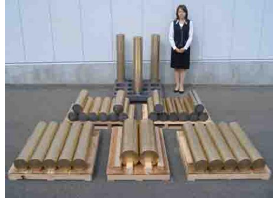
Figure 11.3.7: Typical bronze ingots for Nb 3 Sn wires (Courtesy of Osaka Alloying Works Co., Ltd.). 22
