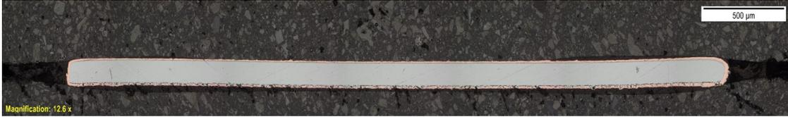
Figure 2.5: Cross-sectional view of SuNAM REBCO CC with 100 microns of 310 SS and 7.5 microns of copper on each side.
