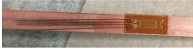
Figure 4.8: REBCO CC with a mounted strain gage.
