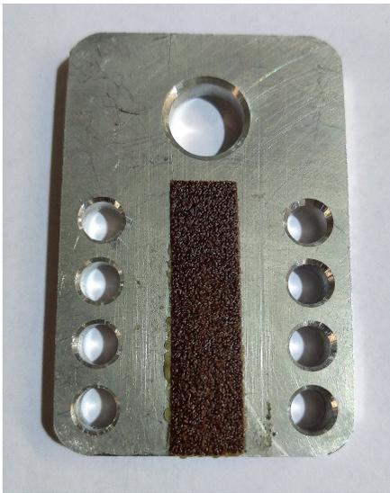
(a) Tension testing grip lined with sandpaper.
