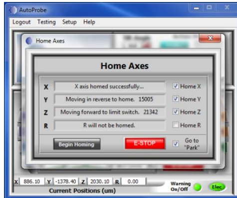
Figure 39 Home Axes window. Image obtained using the AutoProbe® software For more information visit https://www.oxford-instruments.com/
