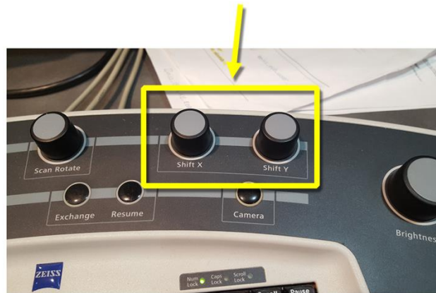
Figure 14 The Beam Shift knobs work for both “E” and “P” images, but adjusting the “E” only is safer. Use these to fine tune your match between the two.
