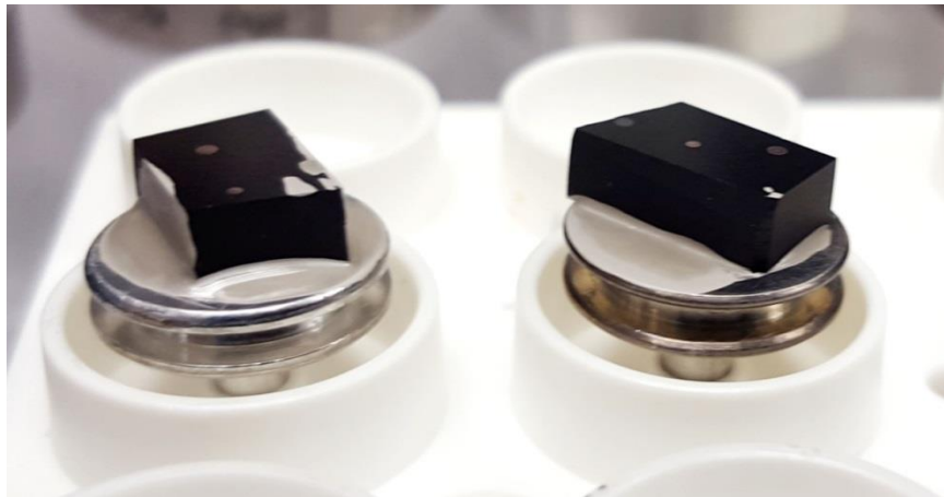
Figure 3 My first FIB samples, extracted from regular metallographic pucks and glued to SEM stubs using silver paint
