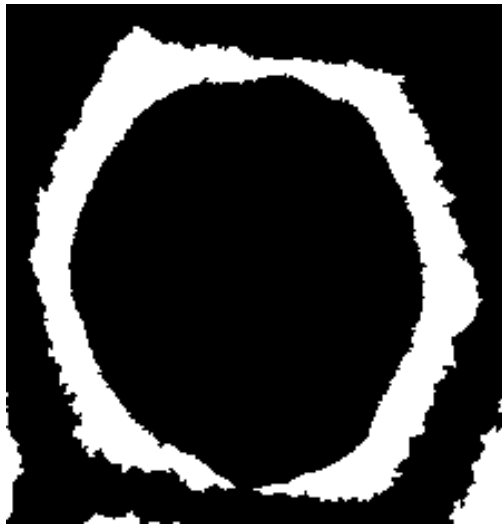
Thresholded unreacted tube (wall) (broken ring)
